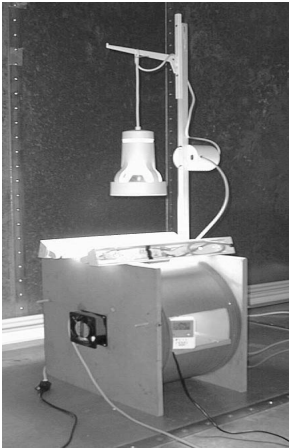
Fig. 2 – View of the Helmholtz bobbins in the experimental chambers; the light sources can be seen above it; Petri dishes can be accessed from both sides.
